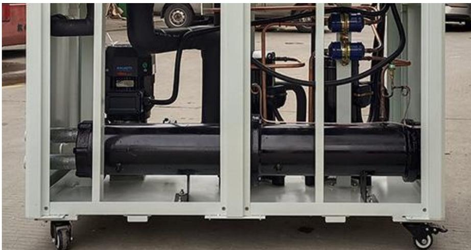
*Shell and tube Condenser for water-cooled PET chiller*
