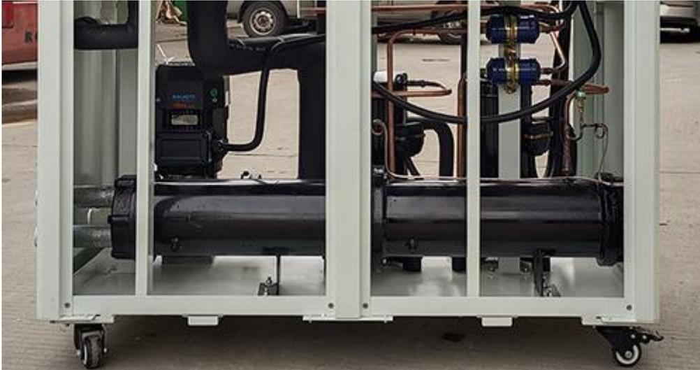
*Shell and tube Condenser for water-cooled MRI chiller*
