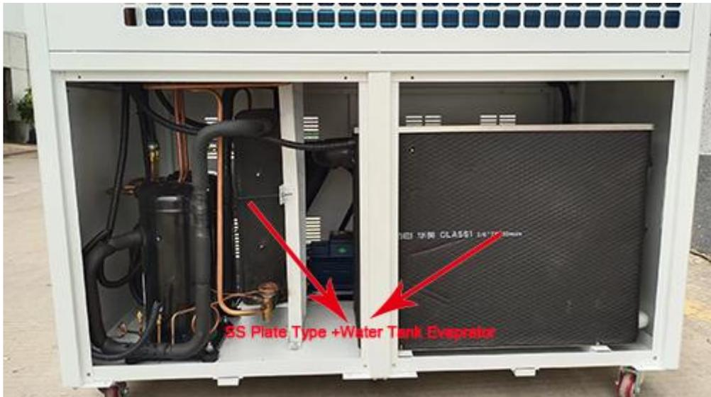
*SS Plate Type+ Water Tank Evaporator*
